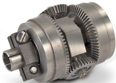
**Fairloc® — A Better Way to Fasten Rotating Components** Engineers have relied on Fairloc® from Stock Drive Products/Sterling Instrument (SDP/SI) for over 50 years. It's a component fastening design that's built into the hub of the part and may be applied to gears, pulleys, couplings, shaft adapters, and other miniature-to-medium-sized (up to 2 in. bore diameter) components.
