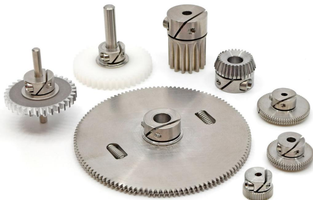
gears and shafts were made of 303 stainless steel. Gear bores were within +/-0.0003 in. of nominal values. Shafts had a maximum surface finish of 16  $\mu$ in. and were within -0.0002 in. of the nominal diameters.
